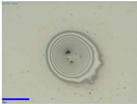
Fig. 5: Reflected light microscopy image of a cluster of IDPs in oil. Scale bar is 80 micrometers.
