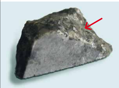
3.1 A 2 x 2 mm area at the indicated position was investigated on this inclined and rough rock sample while the sample was positioned under the microscope exactly as shown in the image.
