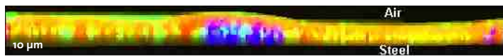
Fig. 5: Cross-section of a drug-delivery coating plus polymer on a stent. Polymer (red), amorphous drug (green), crystalline drug (blue), polymer + amorphous drug (yellow).
